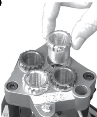
Remove Spline Drive breech lock bushing.
