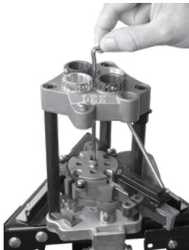
With the carrier at the bottom of the stroke (handle up), install index rod.
