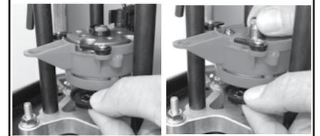
Install driver clutch when no shell plate is installed.
