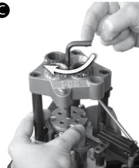
Raise carrier to the mid-stroke position, install shell plate, lightly tighten clockwise with 1/4" hex head wrench.
