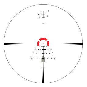
Elevation correction at 600 yards and no wind (.223/5.56mm round)
