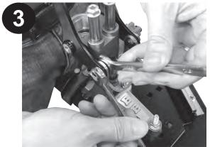
Using two <sup>7</sup>/<sub>16</sub>" or 11mm wrenches, loosen and remove PA4330 crown lock nuts and PA1867 shoulder bolts.
