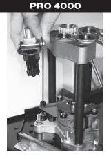
(1) Breech Lock bushing and (1) lock ring are required to utilize Automatic Bullet Feed Product # 90600 and Part # SD4239
