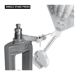
Place finger or thumb **DIRECTLY OVER** "S" or "L" and steer the trigger on to the primer arm, briskly push to dispense primer into cup.
