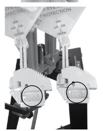
Make sure trough fingers are between and completely engaged with tray latch lugs highlighted below.
