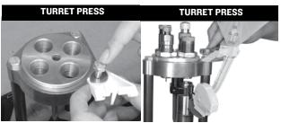
Orientate bracket with feeder installed to primer arm. Tighten Phillips screw.
