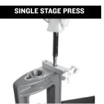
VERIFY appropriate primer arm and trigger assembly are installed.
